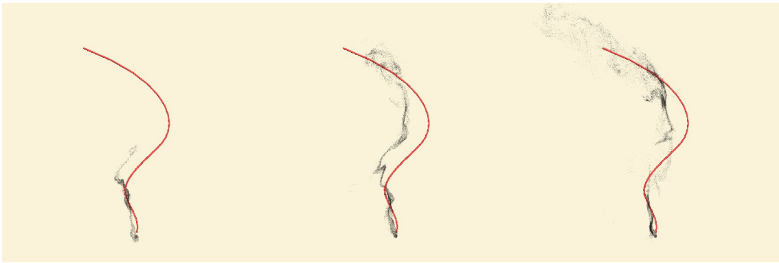
Figure 4: From left to right, the images show particles moving along a flow derived from one spline. The flow consists of eight component fields of different frequencies and amplitudes superimposed for the final result. The algorithm is sufficiently fast and memory-efficient that the fields are calculated on-line during simulation.
